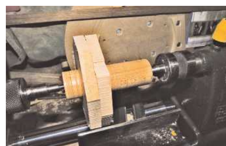
▲ Pic.3 ...pinching them between the drive centre and a tailstock rotating centre
